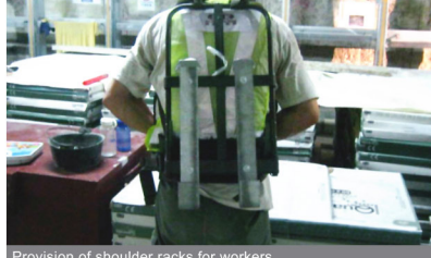
Provision of shoulder racks for workers
